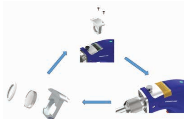
Figure 6-4 Replacement Operation of Focus Lens
