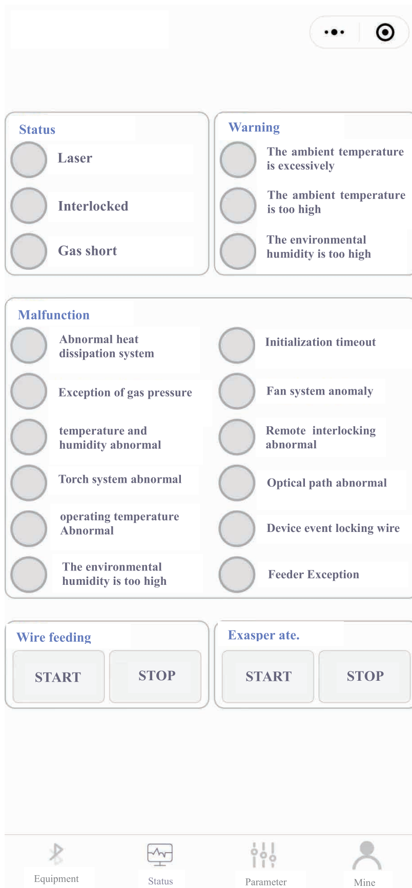
Figure 8-3 Using APP to View Detailed Fault Information
