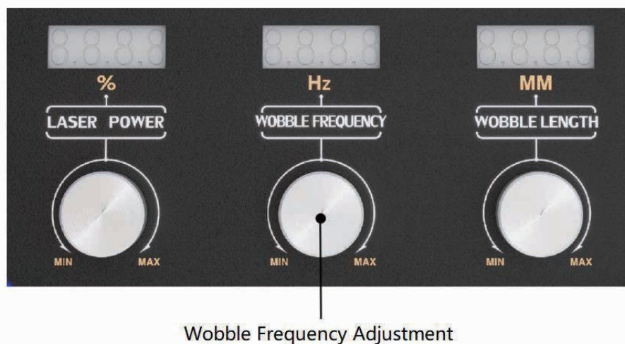
Figure 5-7 Wobble Frequency Adjustment
