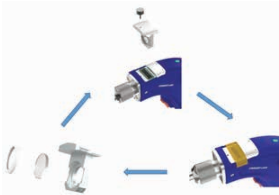
Figure 6-2 Replacement Operation of Protective Lens
