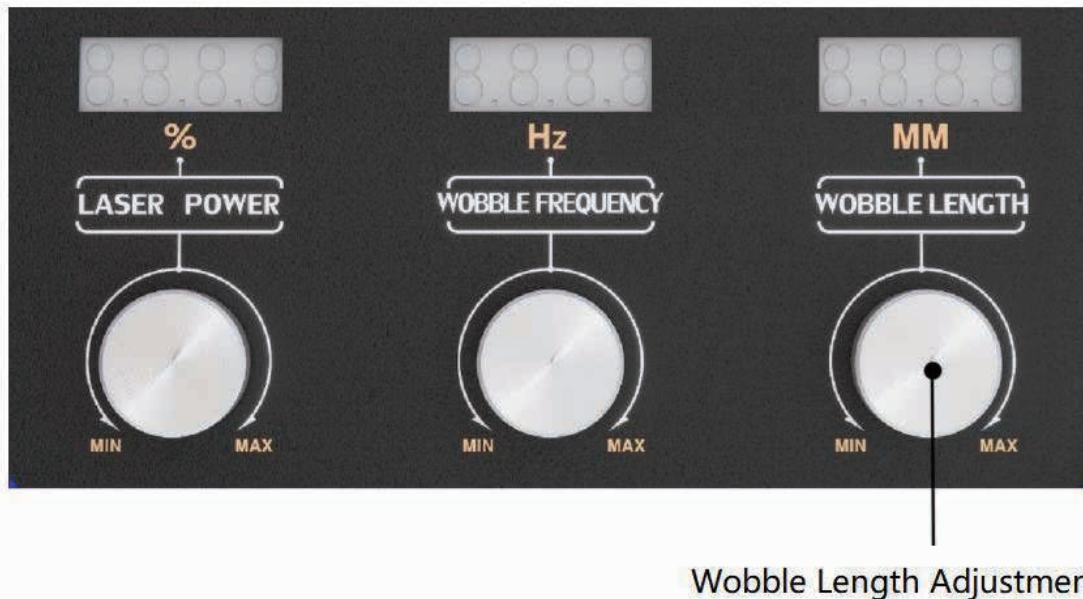
Figure 5-8 Wobble Length Adjustment
